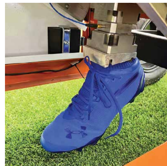
fLEX uses a 3D-printed foot combined with a real cleat to replicate player-surface interaction
